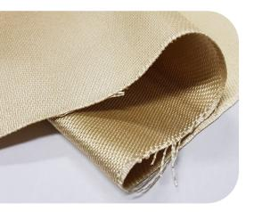
Darco woven **Silica** glass fabrics are woven continuous filament amorphous silica (non-respirable fibre yarns). Silica fabrics are mainly used above 550°C (above E glass rating) for all high temperature applications where the need for thermal insulation and/or protection is required
