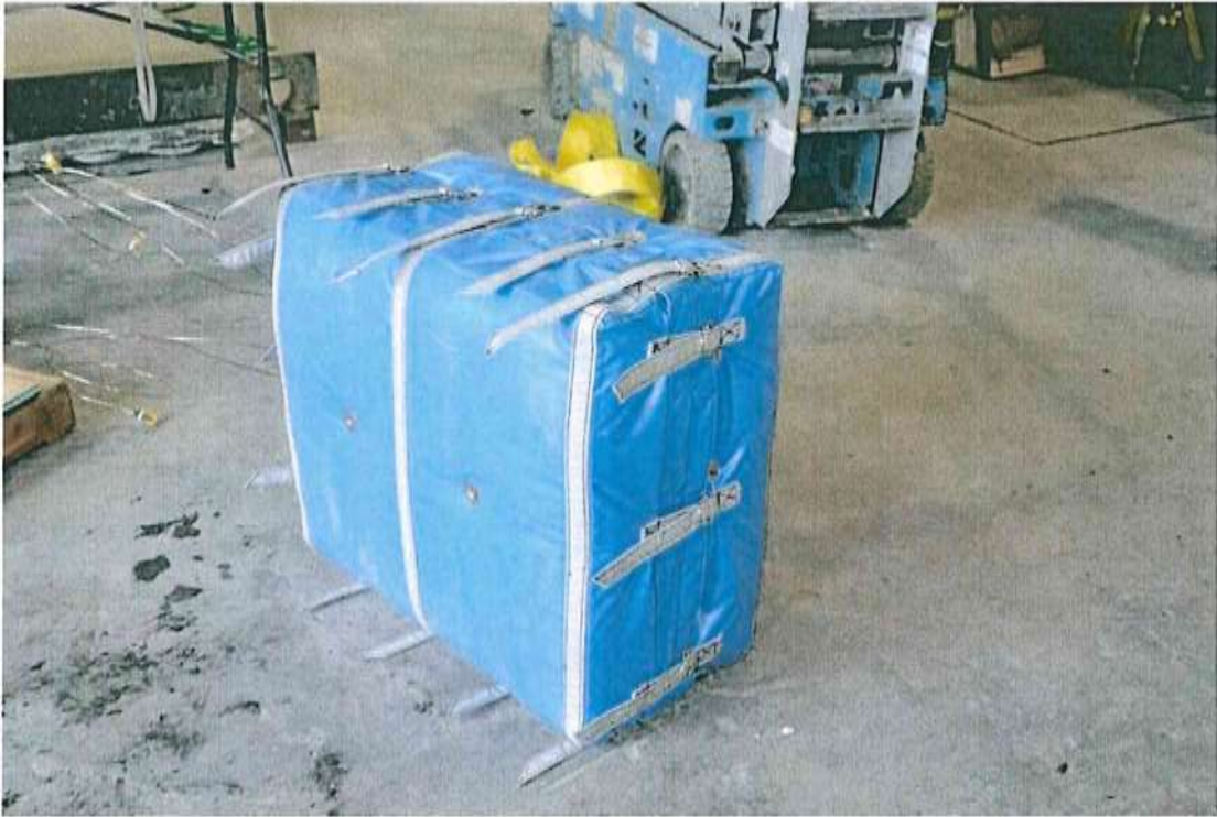
Figure B-1. Assembly Protected with ProSol PFP Fire Jacket System Insulation.
