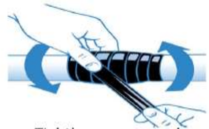
Tightly wrap around damaged pipe
