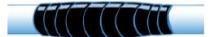
Press loose end down tight to adhere to itself. Pipe is now water and airtight
