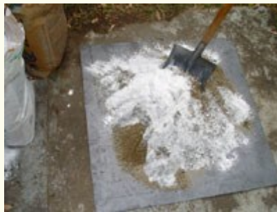
Refractory concrete dry ingredients
