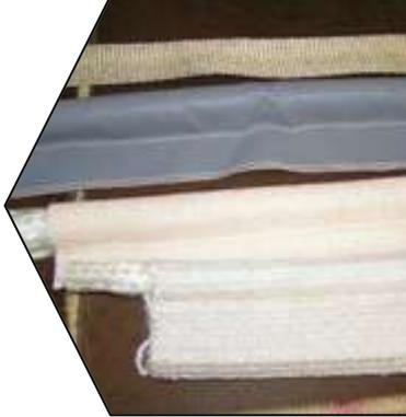
**Ropes** range from fiberglass round and square ropes (braided and knitted types) in various densities and diameters (4 to 50 mm) mainly for door seals in ovens, wood fired heaters, industrial flanges, dampers etc. Ceramic fibre used for higher than 600°C to 1100°C applications.
