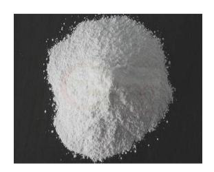
CA80 is manufactured from CA65 or CA70 and œ-Al2O3 micropowder. It is suitable for the preparation of low-cement and ultra-low cement castables. According to customer requirements, in order to adapt to various construction environment changes, some products (CA70A, CA75A and CA80A) with additives have been developed.
