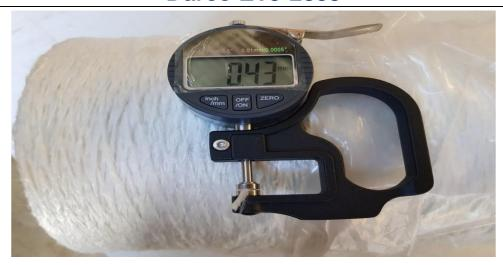
E-glass yarn used for various weaving applications to produce glass fabrics, sleeves, ropes and other finished fiberglass products. Can also be used for silencer packing. Texturised for better sound obsortion.
