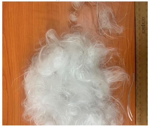
Alternative texturized fiberglass roving can be directly injected into a muffler, plastic bag, and non-woven or winding around the perforated pipe and made into perform parts.
