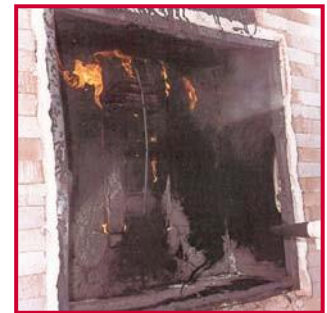
Jet Fire Test to the latest OTI 95 634 standard
