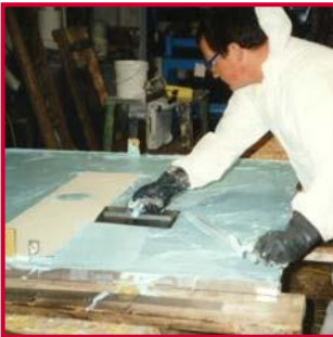
Preparing the Insulant and Intumescent test piece.
