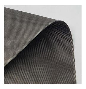
After a 28 day immersion of 5% NaOH solution, the average retention rate for tensile fracture strength is greater than 70%.
